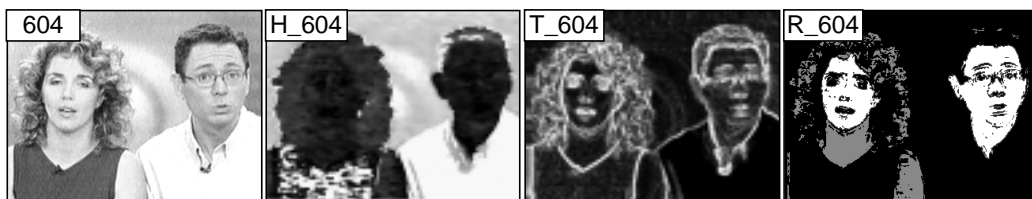
Figure 1: Region searching in HIT maps: input image; hue channel; texture channel; and skin regions found (those verifying size and shape criteria, in white).
