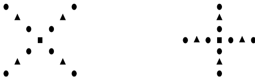
Figure 9: The circles are used to predict the square. For k even, right: reconstruction from level k-2 to k-1 , left: reconstruction from level k-1 to k .
