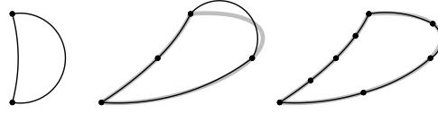
Fig. 4. Transformation of arcs via subdivision. Left: original curve. Center: two divisions per arc, not enough for high curvature sections. Right: four divisions per arc.
