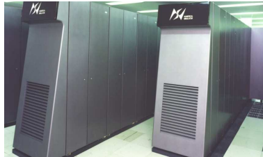
Numerical Wind Tunnel, 167 proc. 170 GFlops National Aerospace Laboratory of Japan nov. 1993 y nov. 1994 a dic. 1995
